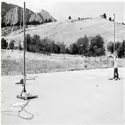
Antenna under test at NIST OATS facility
